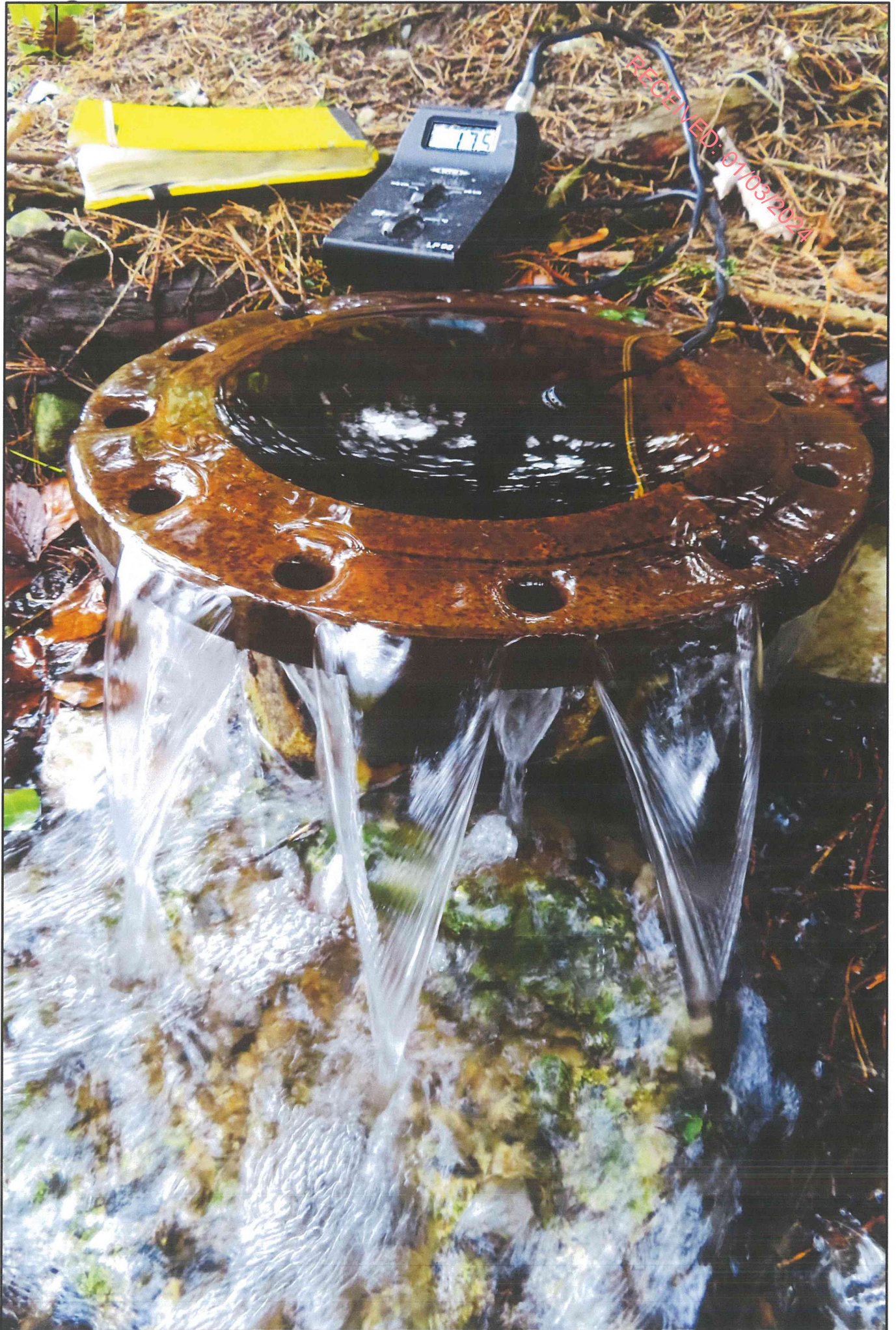
Figure 5.36 Artesian flow from Borehole SG4 at 13.26hr on the 12th February 2021
